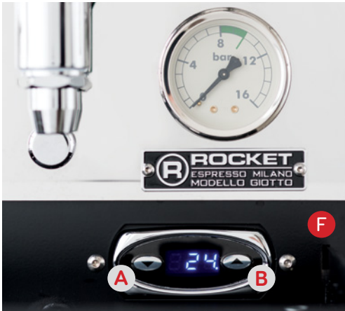
Fig F. The Giotto and Mozzafiato PID display is located directly below the model badge behind the drip tray.
